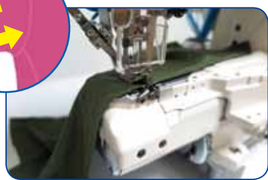
倒骨 Holding-down covering
