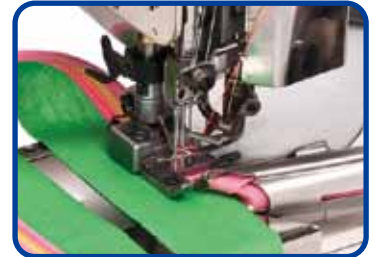
滾邊加雙色線樣品 Decorative stitch for tape binding
