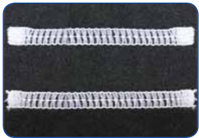
密縫樣式 Sewn sample of condense stitch
